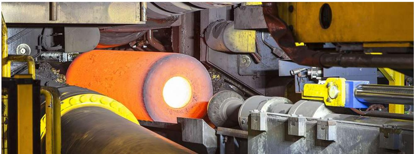
The piercing of solid steel billets and their hot rolling on a mandrel are two key stages in the production of seamless steel tubes. Controlling these processes is crucial to the dimensional and metallurgical quality of the products. With this new tool, Vallourec demonstrates its determination to maintain its highest level of technological expertise and reinforces its position as a global leader.
