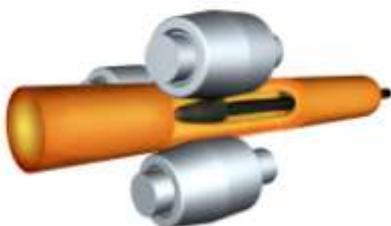
Equipped with three-roll technology, the new piercer is more powerful, enabling it to shape, with outstanding dimensional precision and excellent surface quality, premium tubes designed for the most demanding applications.
